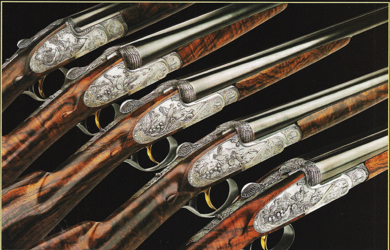
This set of five shotguns includes side-by-sides in (from bottom) 12, 20, 28 and .410 as well as an over/under .410. All actions are scaled to size, and the stocks were made from the same piece of burl wood.
